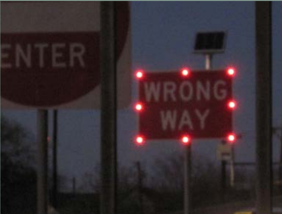
LED ILLUMINATED WRONG WAY SIGN AS SEEN FROM A DISTANCE
