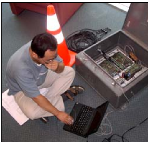
Jeong Hee Nam testing the Campbell Scientific CR10X Data Logger used to capture crack data.
