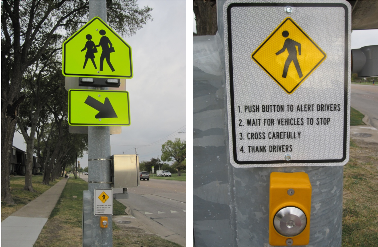
Figure 4. Pedestrian Pushbutton and Instructions for Use of RRFB.
