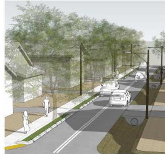
OD-3.3 Rendering of open ditch converted to a standard underground drainage system with a sidewalk and planting strip on top
