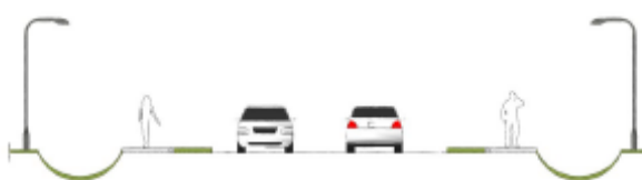
Open ditch next to property line with sidewalk on both sides
