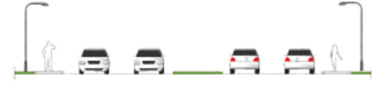
Curb and gutter in a major thoroughfare with unbuffered sidewalks on both sides
